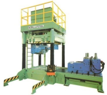
(1) MILLUTENSIL MIL 203 SPOTTING PRESS Workspace: X—79" Y—59"
