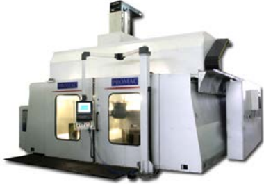
(4) PROMAC SHARAV GVT 3.5 HIGH-SPEED 5-AXIS MACHINING CENTER BLUM LASER TOOL SETTING 15,000 RPM SPINDLE Machine Travel: X—137" Y—86" Z—47"
