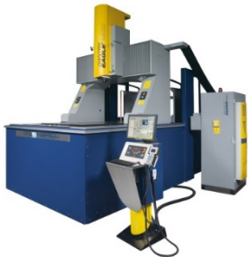
INGERSOLL EAGLE 1400 EDM Machine Travel: X—49.2" Y—92.5" Z—35.4" Table Dimensions: X—59.4" Y—101.2" Z—31.1"
