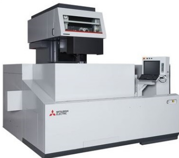
(1) MITSUBISHI MV4800 WIRE EDM V350-V AEII POWER SUPPLY Work Envelope: X—53" Y—43" Z—20" Machine Travel: X—31" Y—24" Z—20"
