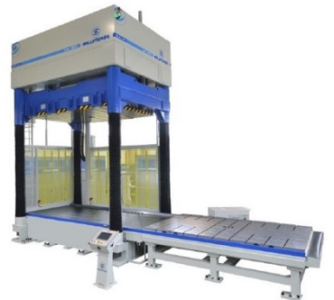
(1) MILLUTENSIL MIL 205 SPOTTING PRESS Workspace: X—79" Y—59"
