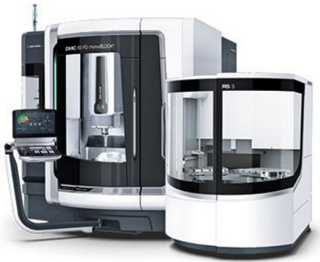
(1) DMG MORI DMC 85 MONOBLOCK HIGH SPEED 5-AXIS VERTICAL MACHINING CENTER 30,000 RPM SPINDLE Machine Travel: X—37" Y—33" Z—25"
