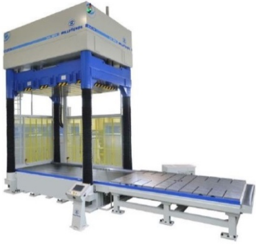
(1) MILLUTENSIL MIL 305 SPOTTING PRESS Workspace: X—118' Y—94"
