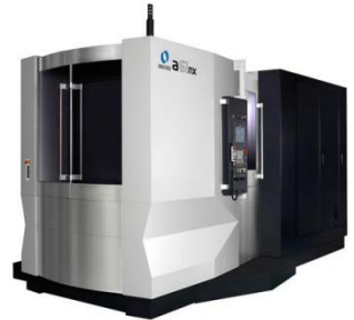
(1) MAKINO A61 HORIZONTAL MACHINING CENTER 14,000 RPM SPINDLE DUAL PALLETS FULL 4 TH AXIS INDEX Machine Travel: X—23" Y—25" Z—25"
