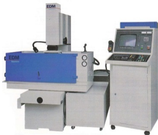
(1) VANGUARD EDM HEIDENHAIN TNC 406 32-BIT Machine Travel: X-18" Y--16" Z—14
