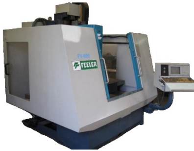
(1) Feeler FV-800 CNC Machining Center Automatic Pallet Changer Machine Travel: X-31" Y-20" Z-18"
